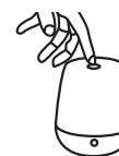
SINGLE TOUCH Turn on the light, select the color temperature, turn off the light.
